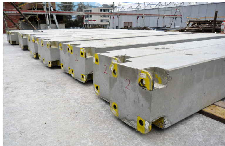
Peikko website image: concrete elements prefabricated with bolt locations.
