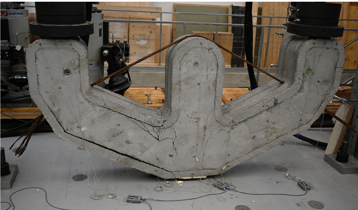
photo taken after the test, once the ULS capacity was deemed to have been reached, showing cracking
