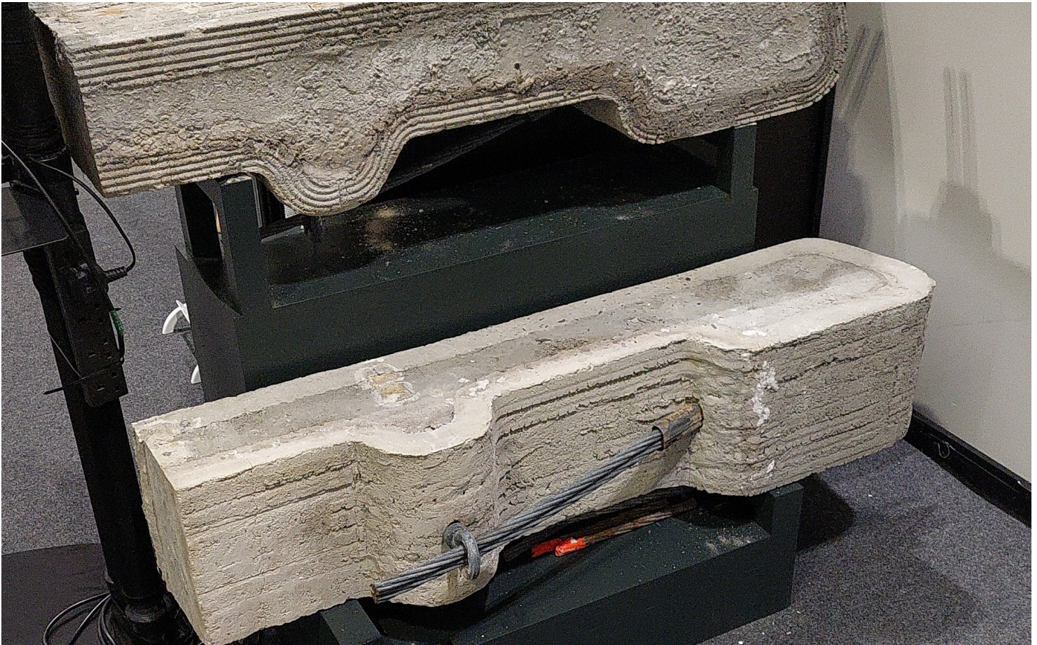
example fire test beam after 132 mins at 1100 deg. C - minimal signs of damage, no spalling or cracking in the 3D printed concrete
