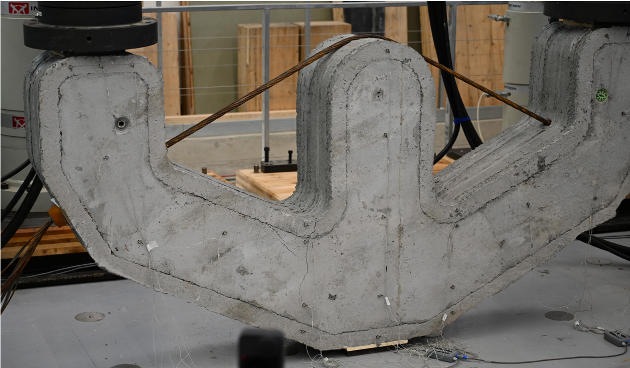
photo taken at 265kN compression force, similar to SLS load level for this design. No damage, minimal cracking.
