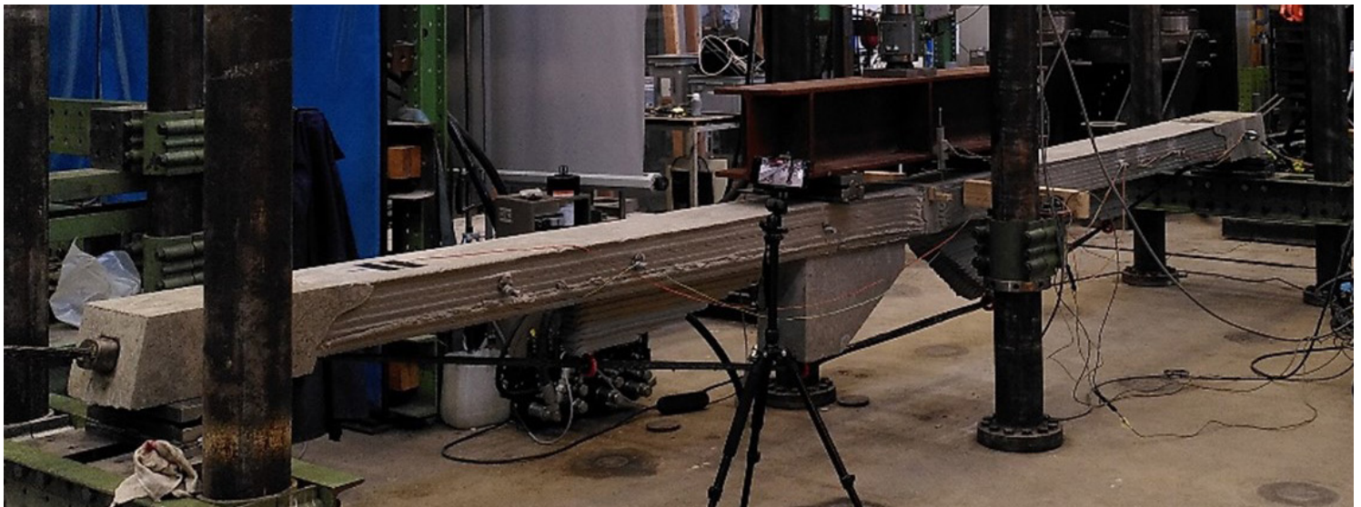
test set-up for 6m long DTU test beams of type MM-01
