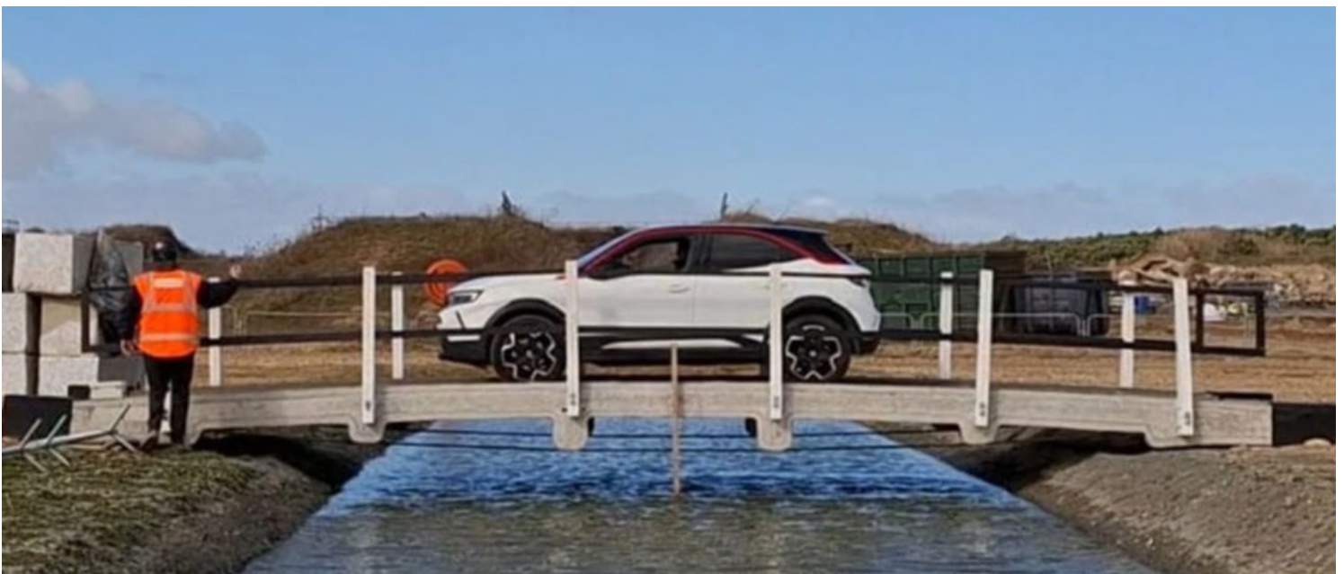
load testing our pilot footbridge in UK
