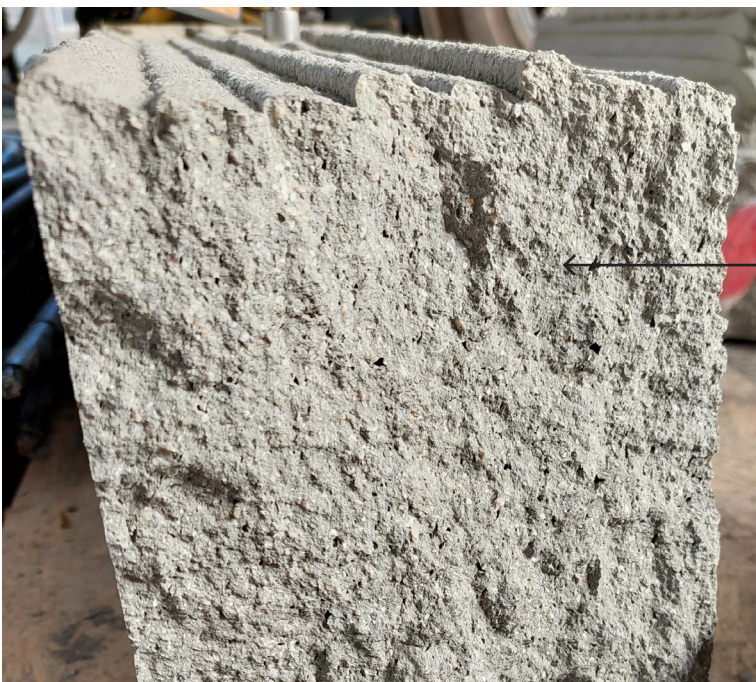
homogeneous concrete texture despite the layering process.
