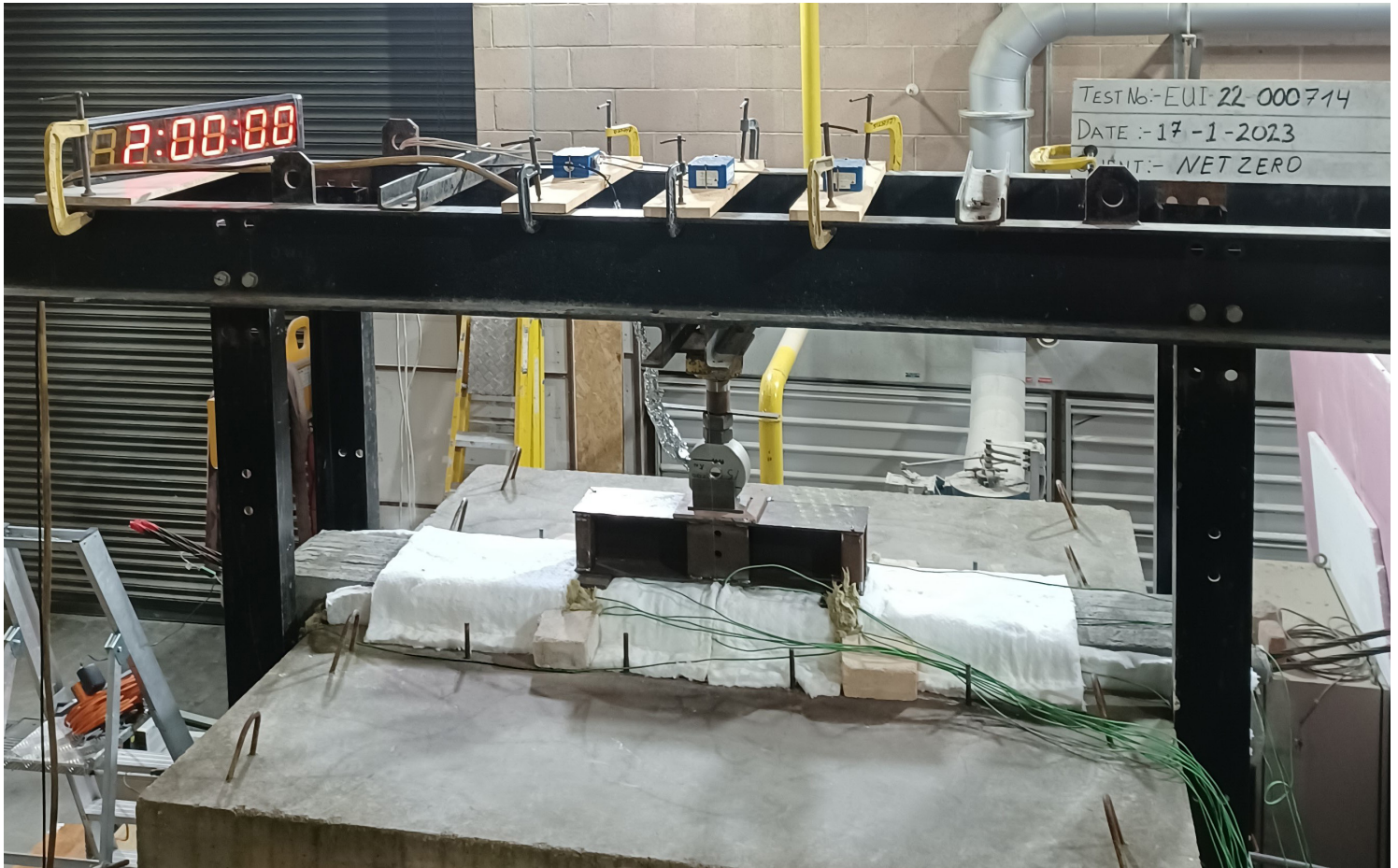
fire test set-up at Efectis, Belfast, showing full integrity at 2hrs fire duration
